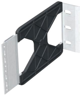
Vertical profiles are connected to the wall brackets with specially designed screws for fixed and flexible points. This allows virtually frictionless movement of the profiles relative to the wall brackets and keeps the profile connected by the fixed point in place. The flexible point makes sure that no additional loads are applied to the substructure by expansion forces exerted by the profile.
