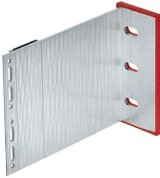
Wall brackets are designed with both fixed and flexible points to allow for thermal expansion of the profile. The fixed point takes the weight of the panels and substructure and the proportional wind loads, while the flexible point only assumes the proportional wind loads.
