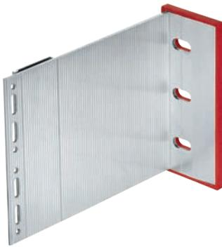
The wall brackets are designed with both fixed and flexible points to allow for thermal expansion of the profile. The fixed point takes the weight of the panels and substructure and the proportional wind loads, while the flexible point only assumes the proportional wind loads.
