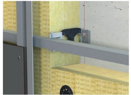
In addition to the pre-assembled connecting screw, the bracket offers an easy and efficient method of installation. Fixed and flexible points are not required as the thermal expansion of the profile is taken up by the flexibility of the bracket. The bracket offers a quick and safe means of fastening – incorrectly installed brackets become a thing of the past.
