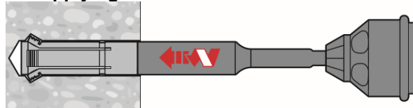
6. Applying hammer drill
