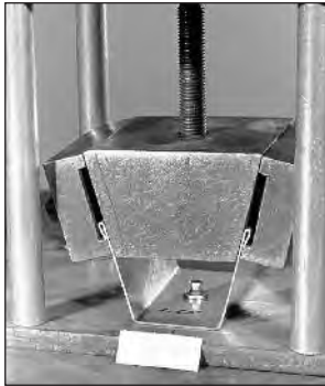
Pull-over test specimen at test start
