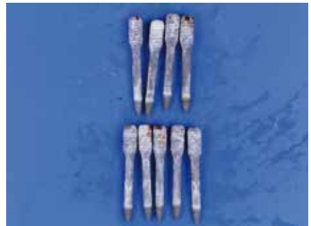
Start of carbon steel corrosion (red rust)
