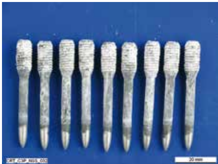
Zinc corrosion (white rust)
