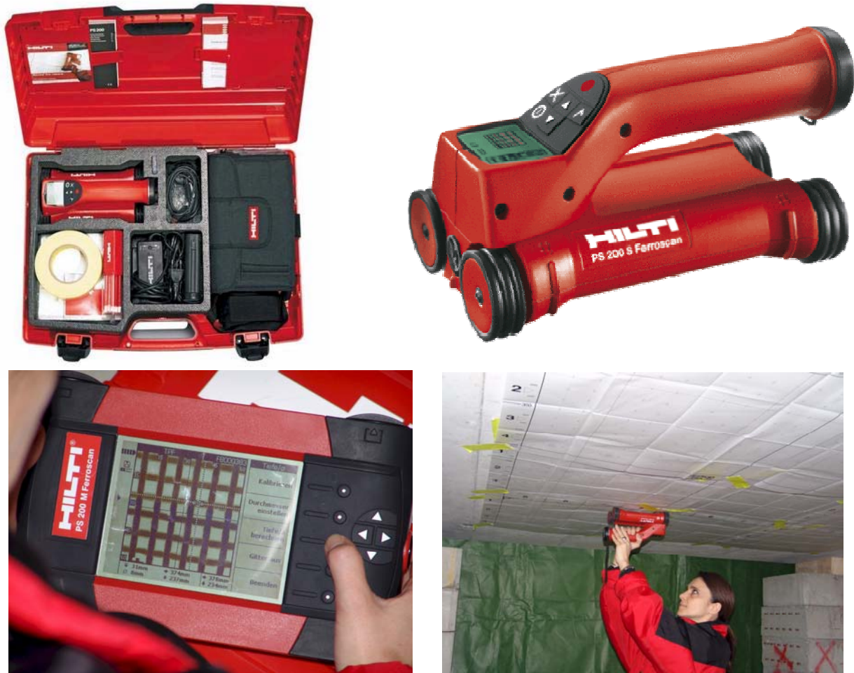
Fig. 12: location of reinforcement with Ferrosan PS200
