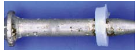
Pitting of a fastener made out of DIN 1.4301 (AISI 304) material (competitor's product).
