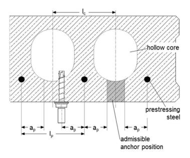
core distance  $I_c \ge 100 \text{ mm}$  prestressing steel  $I_p \ge 100 \text{ mm}$  distance
