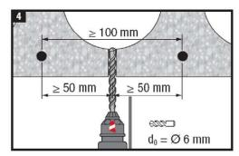
Installation instruction in precast pre-stressed hollow core slabs
