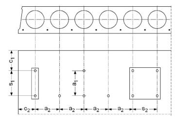
$\begin{array}{ll} \mbox{Minimaler Randabstand} & c_{min} & \geq 100 \mbox{ mm} \\ \\ \mbox{Minimaler Achsabstand} & s_{min} & \geq 100 \mbox{ mm} \end{array}$
