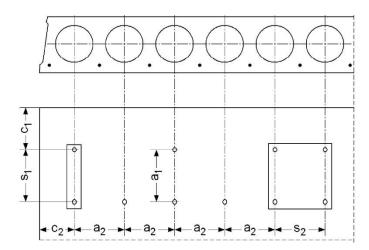
Minimum edge distance  $c_{min}$  ≥ 100 mm Minimum anchor spacing  $s_{min}$  ≥ 100 mm
