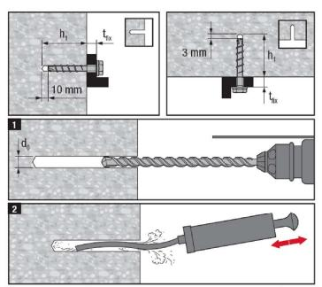
Hole cleaning is not required when 3x ventilation<sup>1)</sup> after drilling is executed and one of the following conditions is fulfilled:
