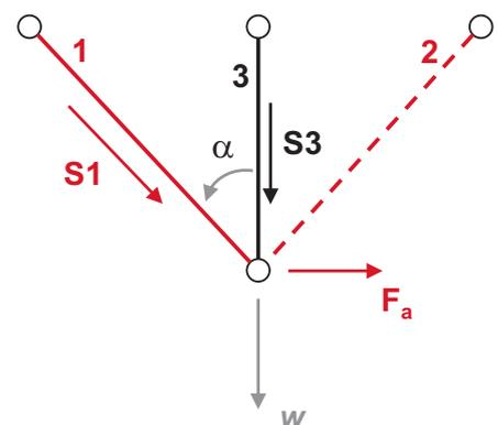
The brace 1 is therefore subject to a tensile force equal to 0.235 kN, considering the horizontal seismic load  $F_a = +0.166$  kN. It's evident that the seismic action, by definition, can act in both directions ( $\pm F_a$ ).
