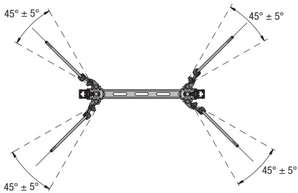
**Top view** – bracing direction on main axis
