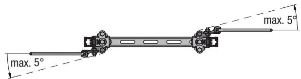
**Top view** – bracing direction on main axis
