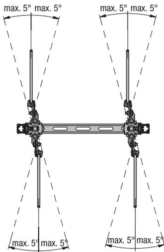
**Top view** – bracing direction on main axis
