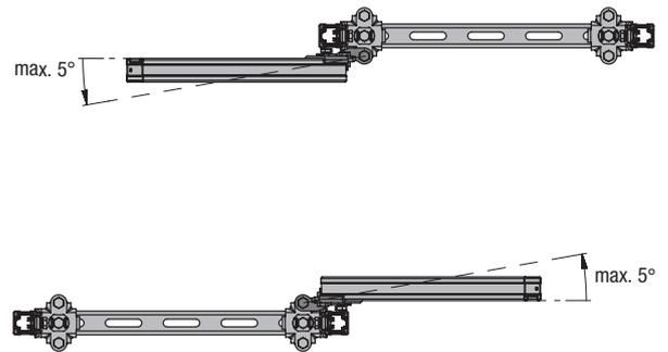
**Top view** – bracing direction on main axis of the pipe run
