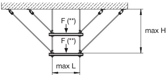
(1) max desing load for each channel level
