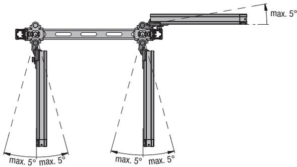
**Top view** – bracing direction on main axis of the pipe run
