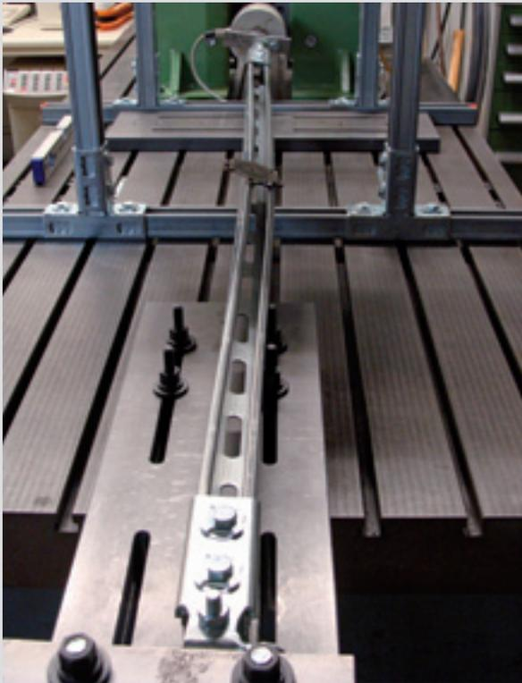
**Fig. H.1** – Compression load test on MQS-ACD component with MQ-41
