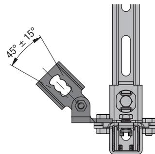
**Side view** – bracing angle on the horizontal level
