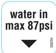
To avoid damage, do not exceed a water pressure of 87 psi / 6 bar.
