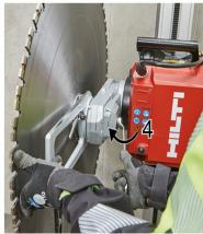
1. Turn the blade guard holder in the direction from which you want to insert the saw blade with inner flange.
