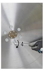
2. Press the flange nut fully into the inner flange.
