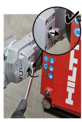
2. Press the flange nut fully into the inner flange (1).
