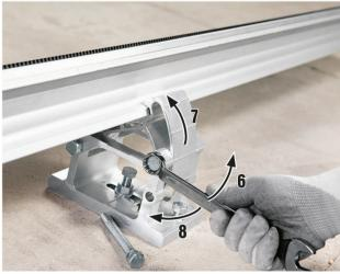
2. Fit the rail onto the rail supports.
