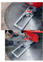
1. Turn the blade guard holder in the direction from which you want to insert the saw blade with inner flange.
